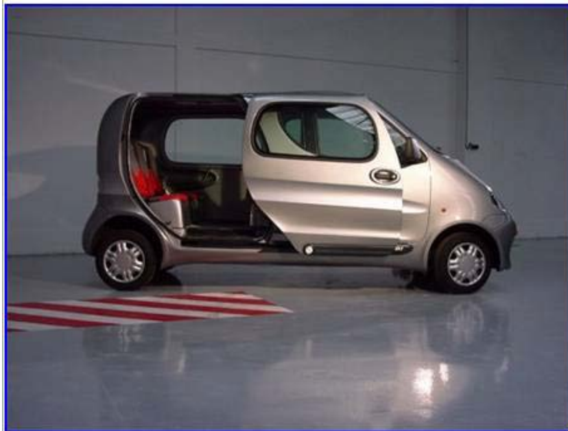
This six-seater taxi, which should be available in India next year, is powered entirely by a tank filled with compressed air.
